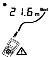
Figure 6.16 Court-circuit du câblage coaxial
