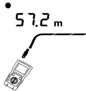
Figure 6.15 Open on Coaxial Cabling
