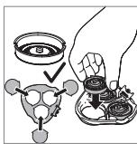
Note: Make sure the notches on both sides of the shaving blades fit exactly onto the notches in the shaving blade holder.
