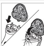
11. Insert the lug of the shaving head into the slot in the top of the appliance.
