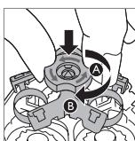
10. Put the retaining frame back into the shaving head and turn the retaining frame lock clockwise.
