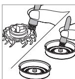
6. Remove the blade from the guard and clean it with the included brush.
