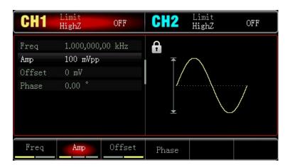
Press Freq to set frequency, enter 900 by numeric keypad, and select parameter unit Hz. Press Amp to set amplitude, enter 100, and select parameter unit mVpp. As the picture shown:
