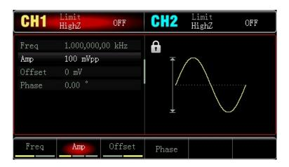
Press Freq to set frequency, enter 10 by numeric keypad, and select parameter unit kHz. Press Amp to set amplitude, enter 100 by numeric keypad, and select parameter unit mV.
