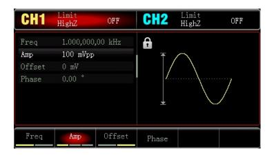
Press Freq to set frequency, enter 2 by numeric keypad, and select parameter unit kHz. Press Amp to set amplitude, enter 1 by numeric keypad, and select parameter unit Vpp.
