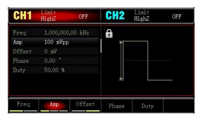
Press Freq to set the frequency, enter 10 by numeric keypad, and select the parameter unit kHz.
