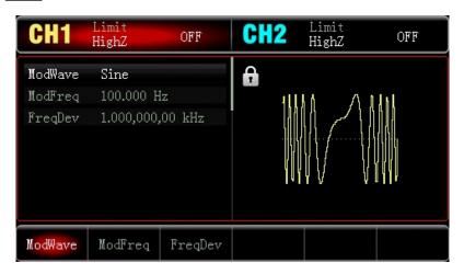
2) Set Modulation Signal Parameter and Waveform
