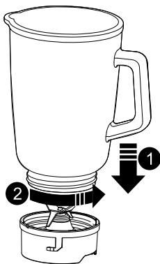
3. Mount the blade assembly in the jar – place the jar over the blade assembly and turn clockwise until locked.
