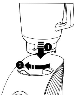
4. Place the jar on the motor unit and turn it clockwise, until it locks in place.
