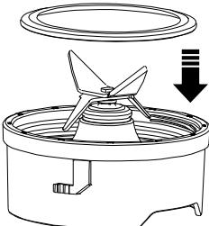
2. Mount the blade unit gasket on the blade assembly.
