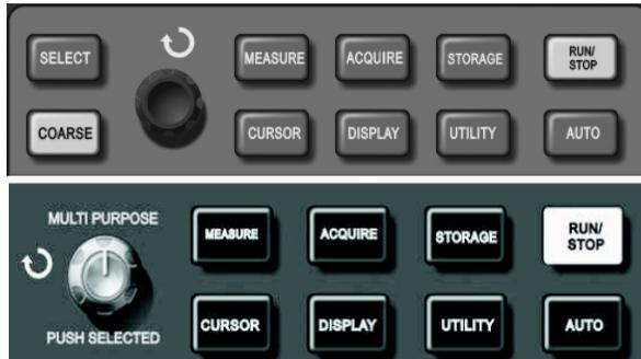
Figure 2-30 Operation/stop key
