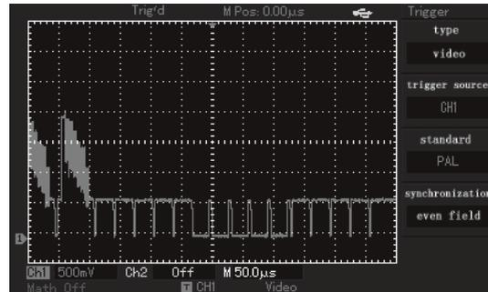
Figure 2–15 Video trigger: Field synchronization
