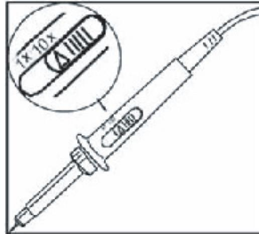
Figure 1—5 Setup of attenuation ratio switch on probe
