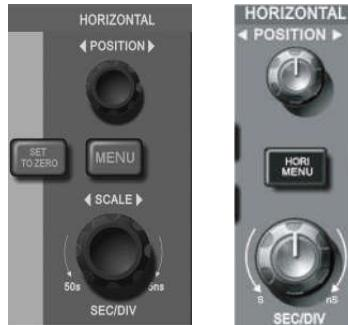
Figure 2-11 Interface of horizontal system
