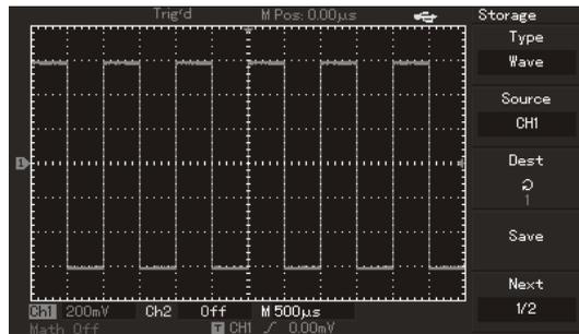
Figure 2-23 Waveform storage
