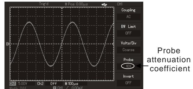
Figure 2-6 Probe attenuation coefficient shown in channel menu
