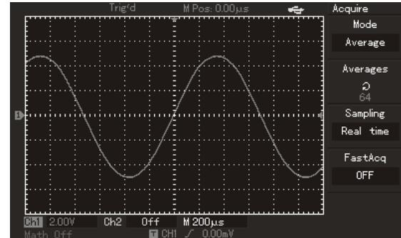
Figure 2-20 Waveform by adopting 32 times of average mode
