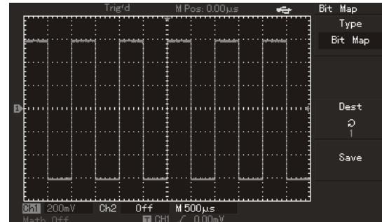
Figure 3-11 Waveform storage
