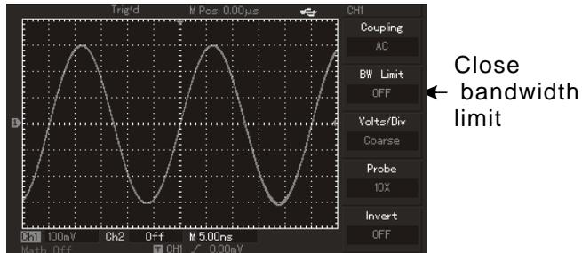
Figure 2-5 Waveform display when opening bandwidth limit
