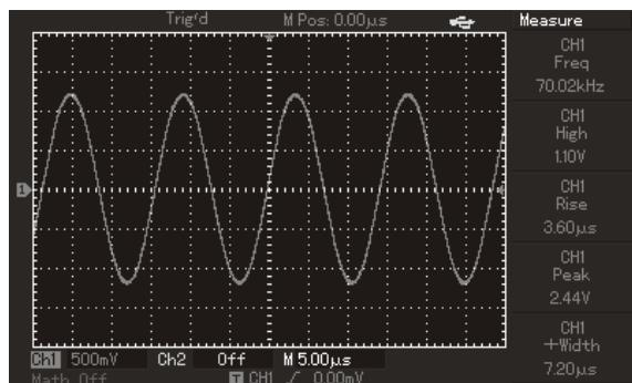
Figure 3-1 Automatic measurement
