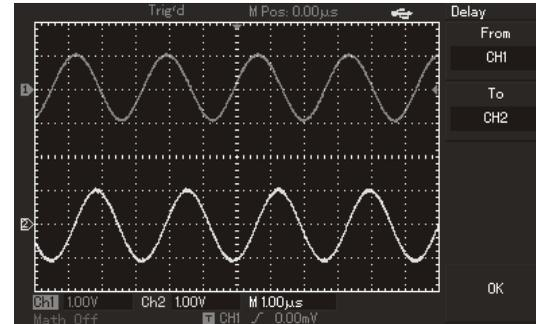
Figure 3-2: Waveform delay
