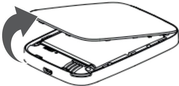
2. Remove battery; Insert the SIM card into SIM card slot.
