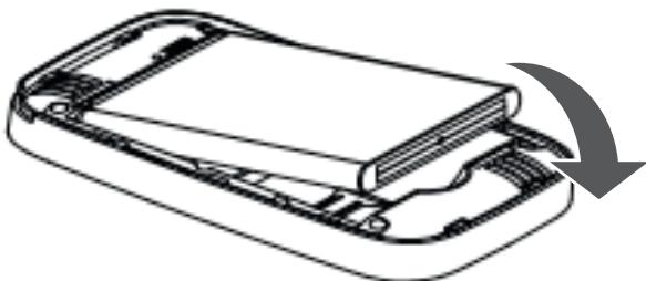
4. Align the back cover with the clip, place the back cover on the device, and close the back cover.
