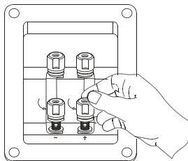
3. Tightening the copper post in clockwise direction, gently pull the wire, and make sure connection firmly.
