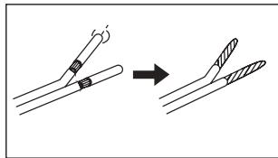
2. Release the copper post in counter clockwise direction, and put the copper wire into the hole.
