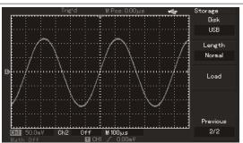
Figure 2-24 Waveform storage by U disk
