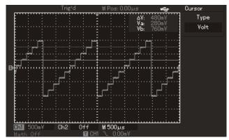
Figure 3-6 Voltage difference of signal by cursor measurement
