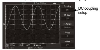
Figure 2-2 Synchronous display of DC and AC components of signal
