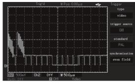
Figure 2—15 Video trigger: Field synchronization
