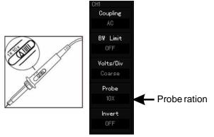
Figure 1-6 Setup of deflection coefficient of probe on digital storage oscillograph
