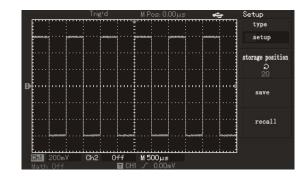
Figure 3-10 Saving setup interface
