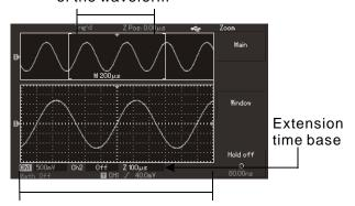
Horizontally extended part of the waveform Figure 2—12 Screen display under view window extension (As shown in above figure), it can be divided into 2 display areas under extension time base. Original waveform is displayed for upper part. Selected area can move horizontally by rotating horizontal POSITION knob or increase or decrease by rotating horizontal SCALE knob.
