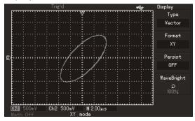
Figure 2-13 Waveform display under X-Y mode
