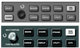
Figure 2—18 Function key of sampling system User can use ACQUIRE key to pop out sampling setup menu so as to adjust sampling mode by control button shown in the menu.
