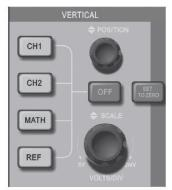
Figure 3-13 Vertical control panel of 5.7-inch screen
