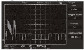
Figure 3-8 Trigger of video field
