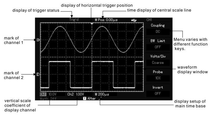
Interface display diagram of digital storage oscillograph (i.e. UTD2000L series)
