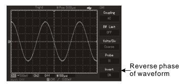
Figure 2—9 Setup of reverse phase of vertical channel
