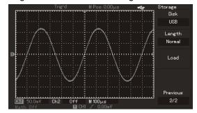
Figure 3-12 Waveform storage by U-disk
