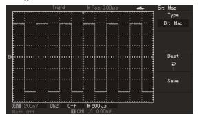
Figure 3-11 Waveform storage
