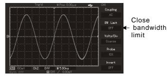
Figure 2—5Waveform display when opening bandwidth limit
