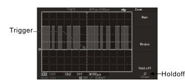
Figure 2—17 Hold off used for synchronization of complex waveform
