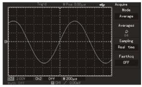
Figure 2-20 Waveform by adopting 32 times of average mode Note :
