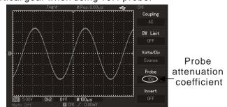
Figure 2—6 Probe attenuation coefficient shown in channel menu
