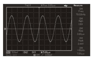
Figure 3-1 Automatic measurement
