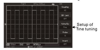
Figure 2—7 Coarse tuning and fine tuning of vertical deflection coefficient
