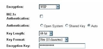
802.1x Authentication: Check the box to enable the 802.1x authentication.
